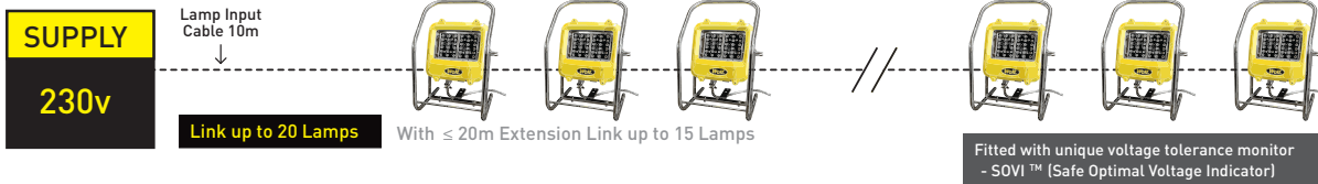
LinkEx™ LED Emergency Temporary Luminaire Linkable with ATX plug/socket, SY 5m 2.5mm 2 cable, input 230V (e.g. LX-400EHA230/T4/SY5)
