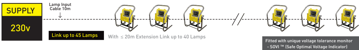
LinkEx™ LED WF-250XL Floodlite Linkable 10m with ATX plug/socket, SY 10m 2.5mm 2 cable, input 230V (e.g. WF-250XL/SY10/ATX230/LINK)
