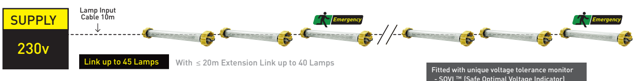
LinkEx™ LED Emergency Temporary Luminaire Linkable with ATX plug/socket, SY 5m 2.5mm 2 cable, input 230V (e.g. LX-400EHA230/T4/SY5)
