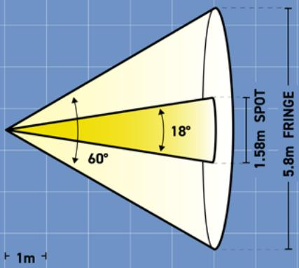
Spot Beam, approximately 18°, with a flood, approximately 60°, of lower level fringe light.
