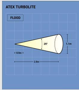
**A-TL45C - Floodlight** Flood Beam **(approx 25°)** Peak luminous intensity at 5m **950lux**
